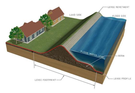
Figure 8-2: Example of additional levee reinforcement to prevent flooding within inland areas.
