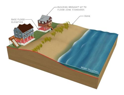
*Figure 8-4: Example of elevated shoreline structures to prevent damage during flood events.*
