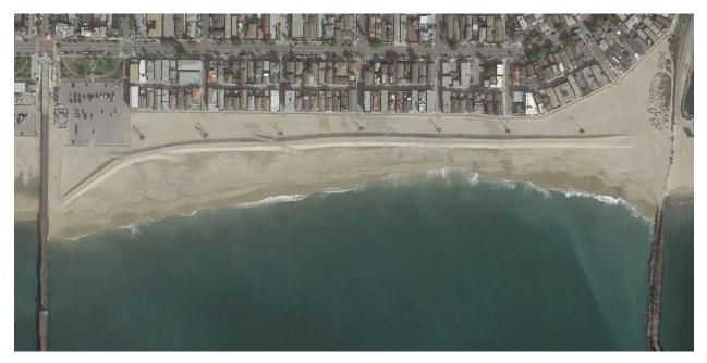
Figure 2-5: Satellite image of sand dike construction in winter 2017. (Photo credit Google Earth)
