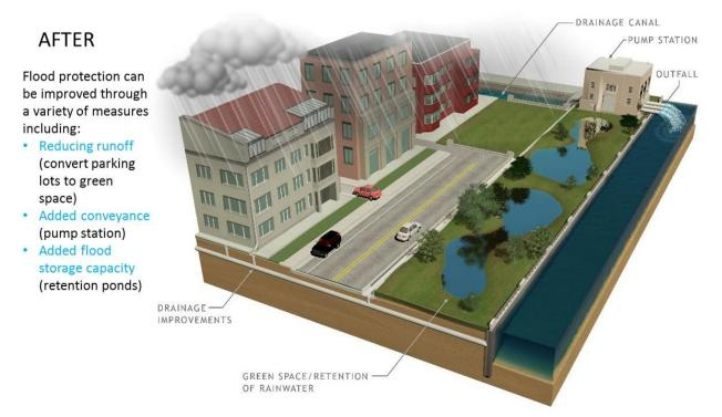
Figure 8-5: Example of drainage improvements to reduce flooding (U.S. Army Corps of Engineers, 2015a).
