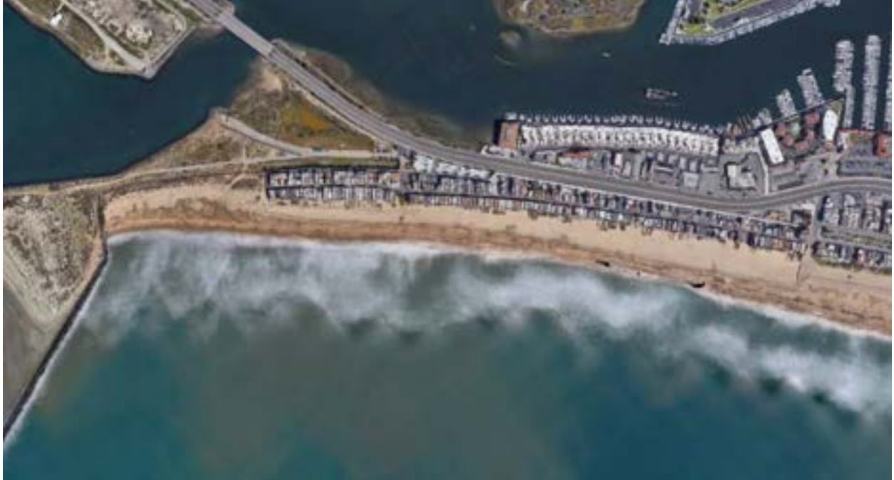
Figure 2-8: 2018 imagery of shoreline downcoast of Anaheim Bay showing significant loss of beach area from previous nourishment event.
