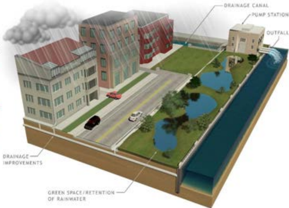
Figure 8-5: Example of drainage improvements to reduce flooding (U.S. Army Corps of Engineers, 2015a).
