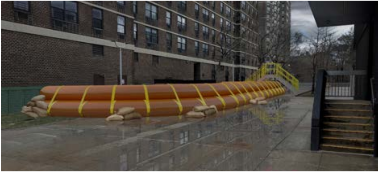
Figure 8-14: Conceptual design of water-filled barriers that can be rapidly deployed around threatened structures. (Visualization produced by M&N for NYCEDC, Interim Flood Protection Citywide)
