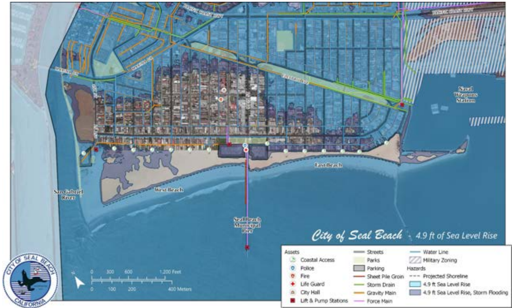
Figure A-8: 4.9ft SLR hazards, Seal Beach waterfront.
