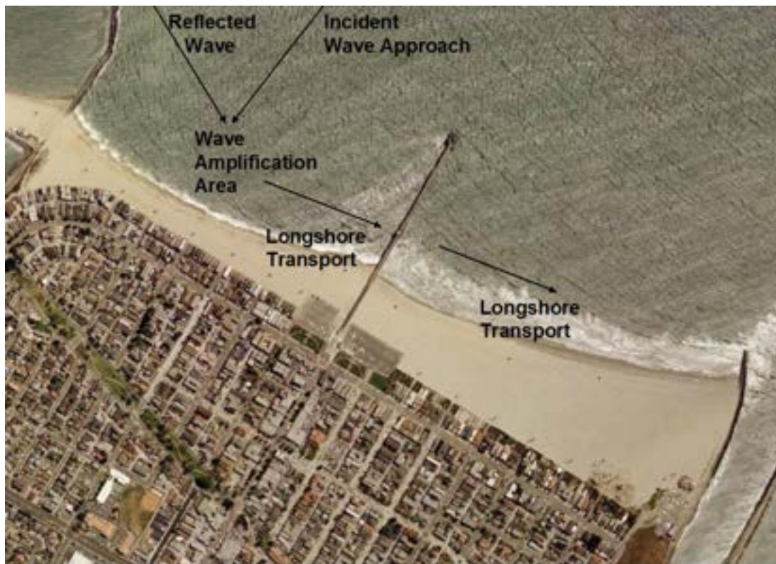
Figure 2-4: Longshore sediment transport patterns along Seal Beach.
