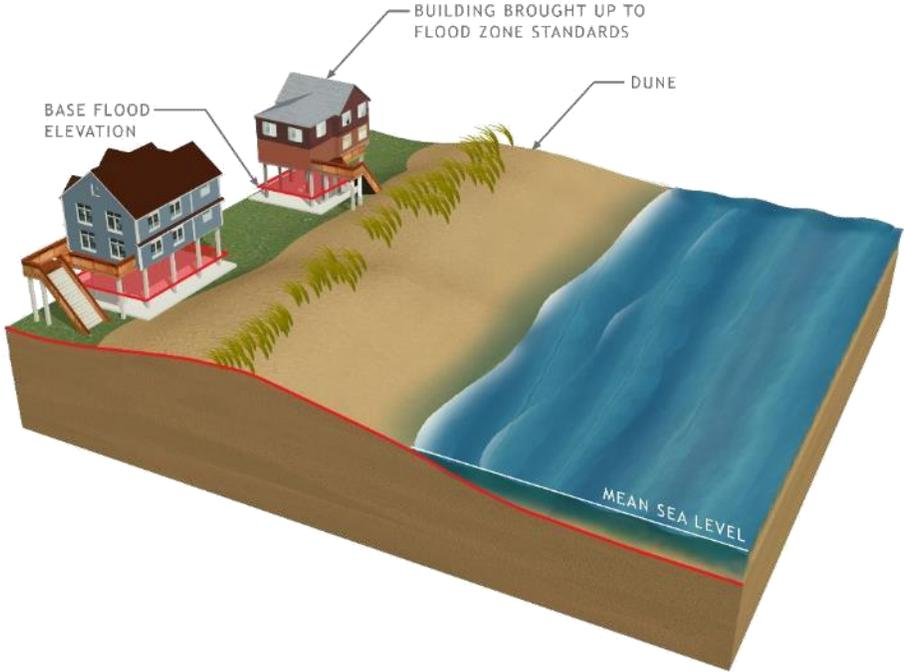
Figure 8-4: Example of elevated shoreline structures to prevent damage during flood events.
