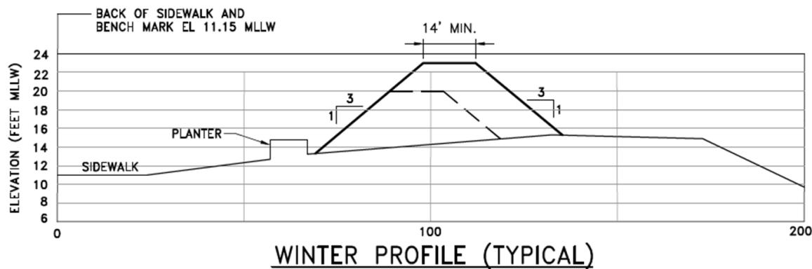
Figure 2-6: Typical cross section of winter dike.
