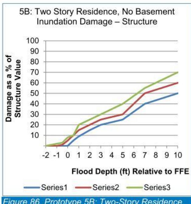
Figure 86. Prototype 5B: Two-Story Residence, No Basement, Inundation Damage – Structure
